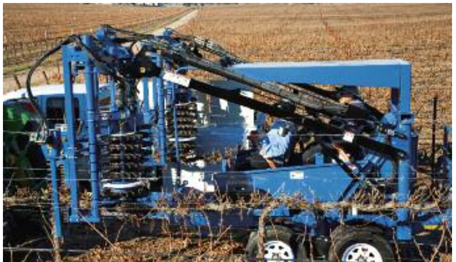
Mechanized pruning with Korvan 2220 tow-behind tool carrier at Red Hills Vineyard (Creston, CA).
