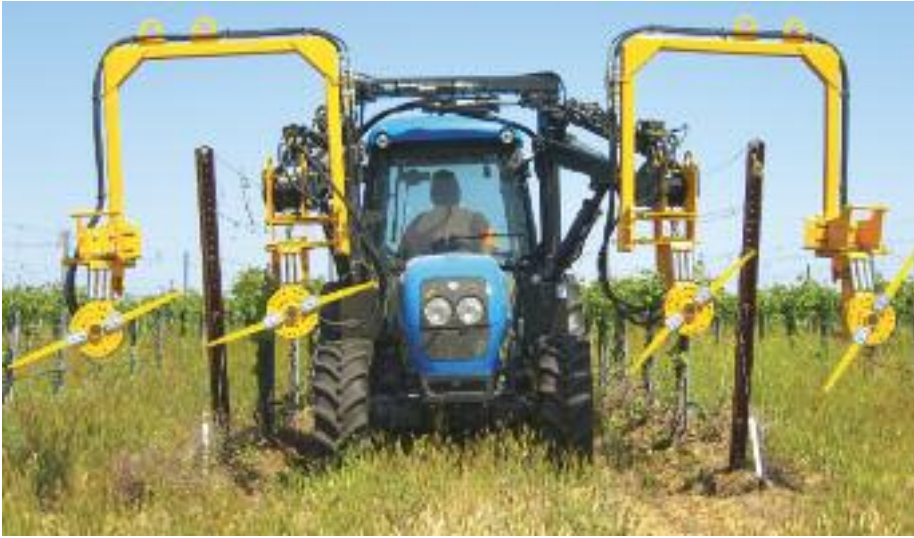
A Korvan 1220 tool carrier with a rotary-paddle attachment is used to remove approximately 40% of the shoots from Cabernet Sauvignon vines (Ste. Michelle Wine Estates, Washington).
