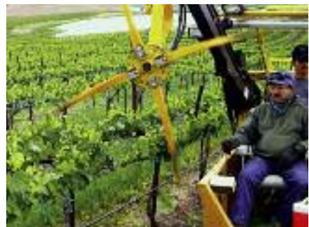
Mechanized shoot-thinning with Korvan 2220 tow-behind tool carrier at French Camp Vineyards (Shandon, CA).
