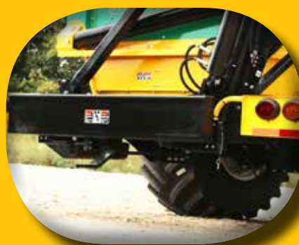
Heavy duty rear bumper: Available with a rugged drawbar for additional towing capacity
