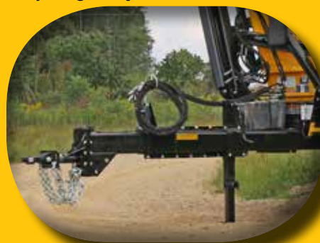
Adjustable pole: Choice of short or long pole. Both are designed to make easy length adjustments
