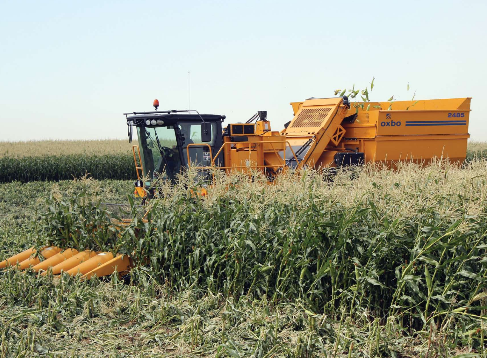
Redesigned dump box: Dump at any height. Simplified design eliminates bell-cranks, links, and cables to reduce maintenance. Large size reduces amount of required stops to unload
