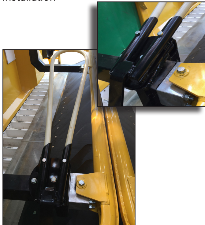
Rod Correctly Mounted in a Standard Oxbo Trunk Shaker.
